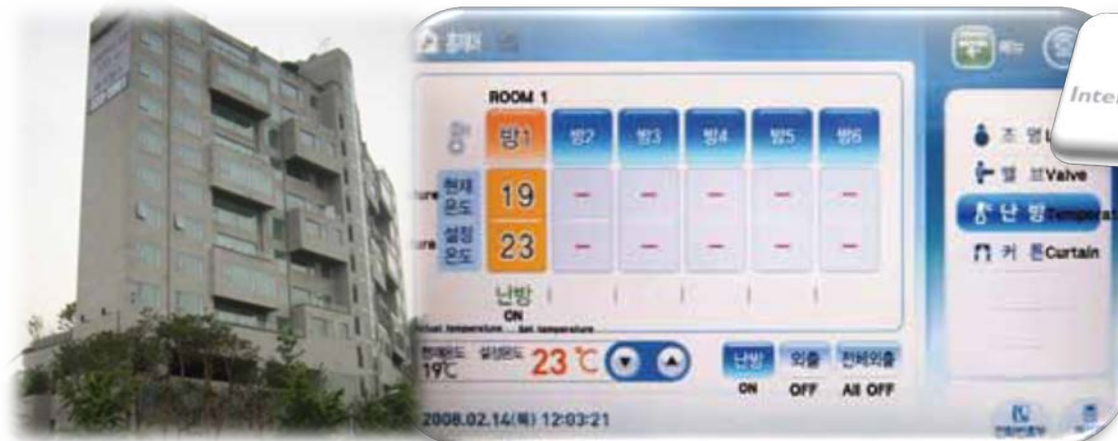
World standard in uniform design for apartment building in Seoul. Comfortable operation of KNX functions by a central touch panel: for example, menus for heating, curtains and lighting
